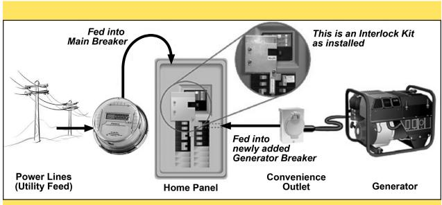
A diagram of a mechanical interlock switch that was recently installed at GELD
